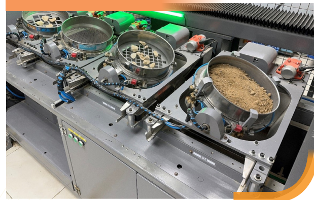
Automated Soil Proctor Compaction Testing System completely eliminates manual labour work, such as manual handling of heavy soil materials.
