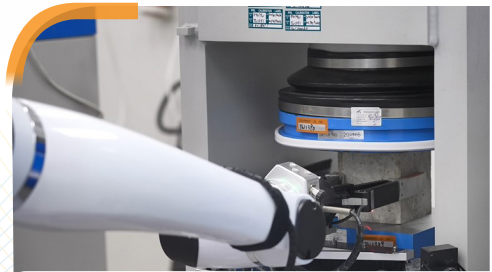
Automated Concrete Cube Testing System fully automates the entire process from concrete cube curing to testing, significantly improving OSH by minimising manual handling of repetitive tasks.
