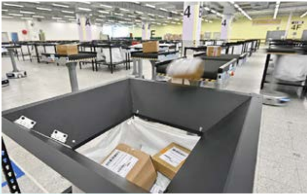
Sorting robots transport the packets to their respective unloading fittings according to the information recorded in the system.
