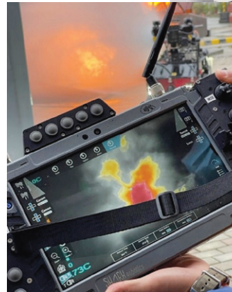
Firefighting robot operator using thermal imaging display function at remote control to monitor fire situation and carry out firefighting work.
