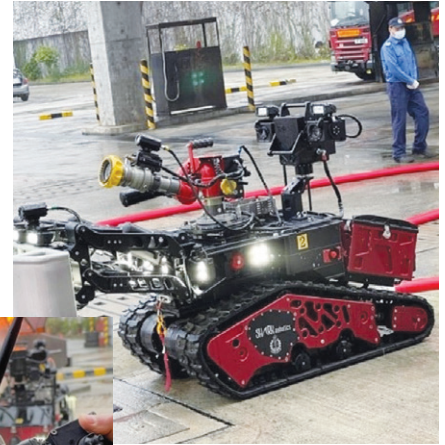
Firefighting robot operator using thermal imaging display function at remote control to monitor fire situation and carry out firefighting work.
