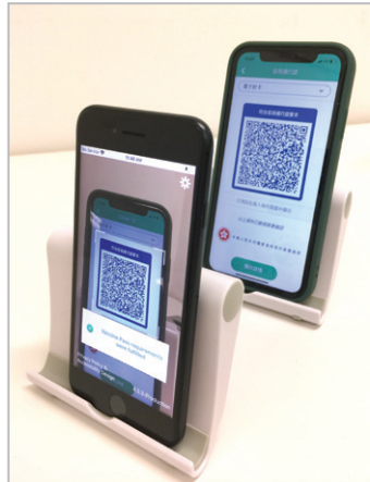
Simple set-up of using rear camera to scan QR code.
