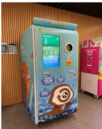
*Reverse vending machine at CGO to collect used plastic beverage containers*
